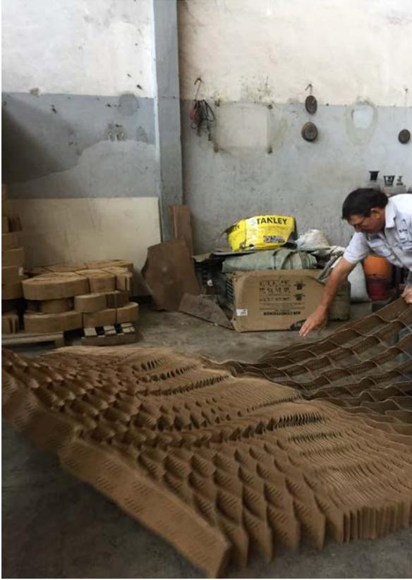
**Geocells (same used in construction of Beira WTRC).**
